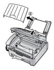
Remove the recording paper (①), then remove the drum and toner unit (②) to allow the jammed paper (③) to pull free from the rear cabinet.
